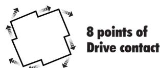
The LOX drive technology was created to solve the problems of all the other recess types. The sure-fit bit and 8 points of contact create a unique torque maximization that utilizes the full power of your power tool. The LOX recess requires much less effort to drive. The recess is much less likely to strip out as compared to other recesses. It is the only technology that gives you extended bit life and gives consistent results drive after drive.
